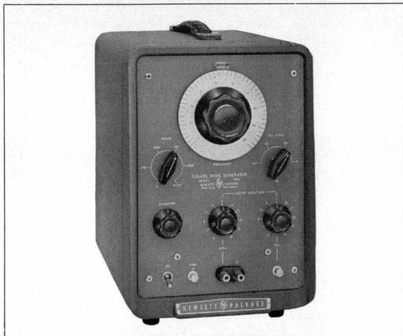
Fig. 1. New -hp- Model 211A Square Wave Generator operates from 1 cps to 1 megacycle, has only 20 millimicroseconds rise time from fast output. A second output provides up to 55 volts peak-to-peak.
